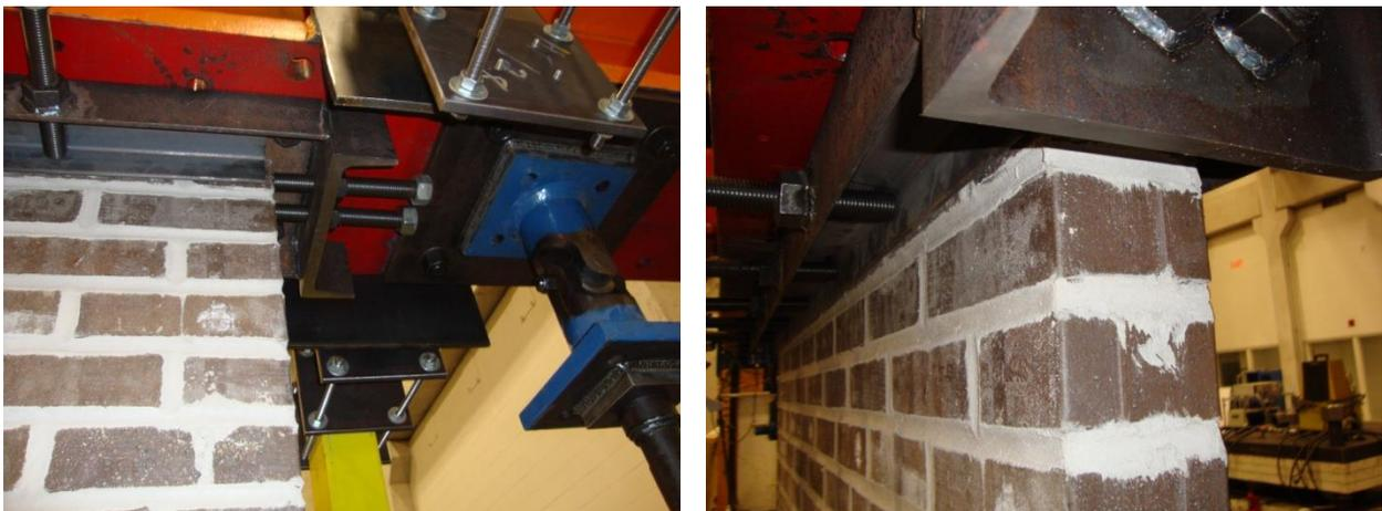
**Figure 8-3. Boundary condition for the top plane of the walls**
