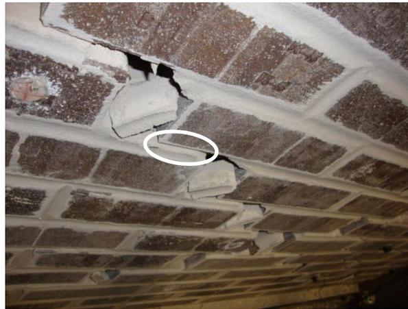
**Figure 8-67. Out-of-plane gap in the joints at the end of the test**
