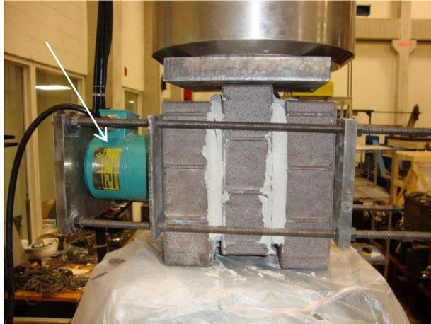
**Figure 8-7. Test setup for measuring the shear properties**
