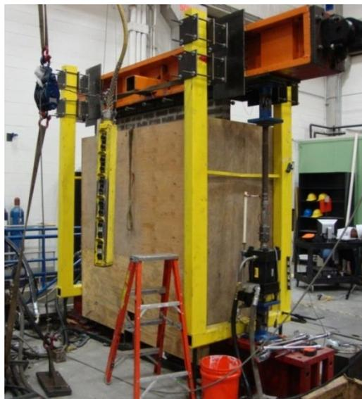
**Figure 8-56. Test set-up for out-of-plane load**
