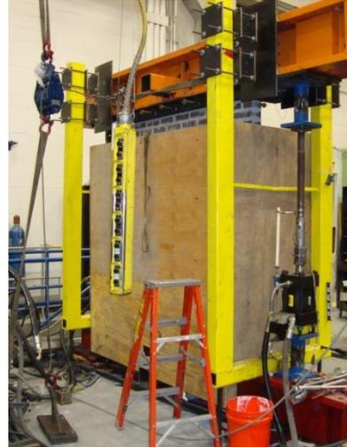
(b) Out-of-plane loading set-up
