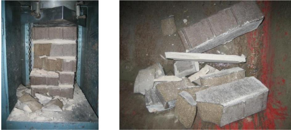
**Figure 8-13. A damaged masonry prism after compression test**
