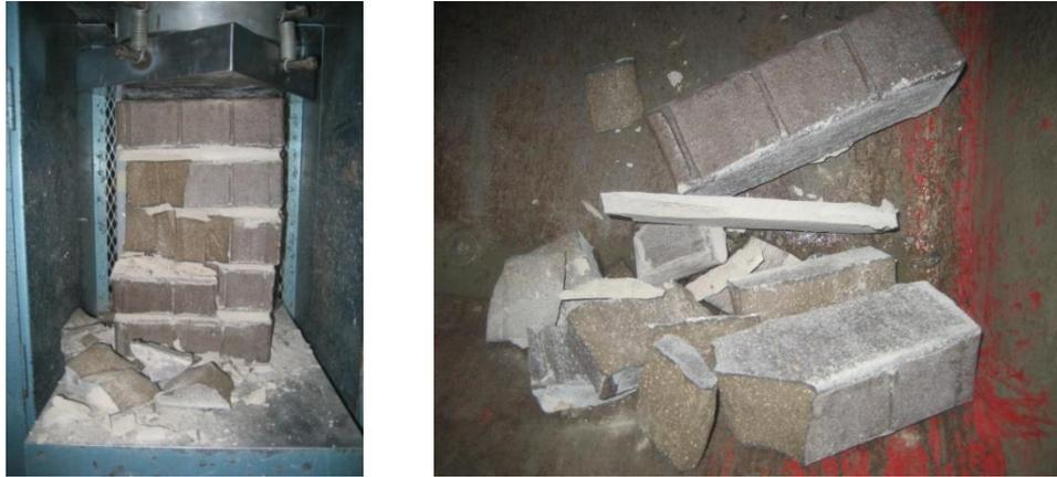
**Figure 5-11. The damaged specimen after compression test**
