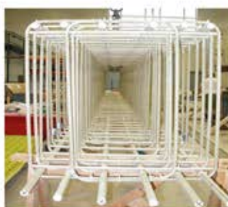
Carbon &amp; glass polymer rebar with epoxy and polyester resin
