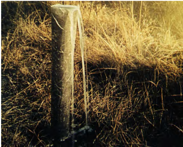
Figure 9.3 Example of discharge from a prefabricated vertical drain (PVD) drain.
