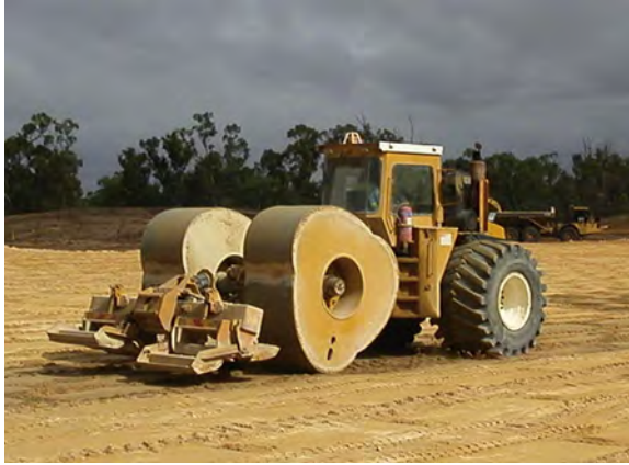
Figure 5.11 Impact roller. Courtesy of Landpac Technologies.
