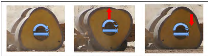
Figure 5.12 Dynamic action of the impact drum. Courtesy of Landpac Technologies.
