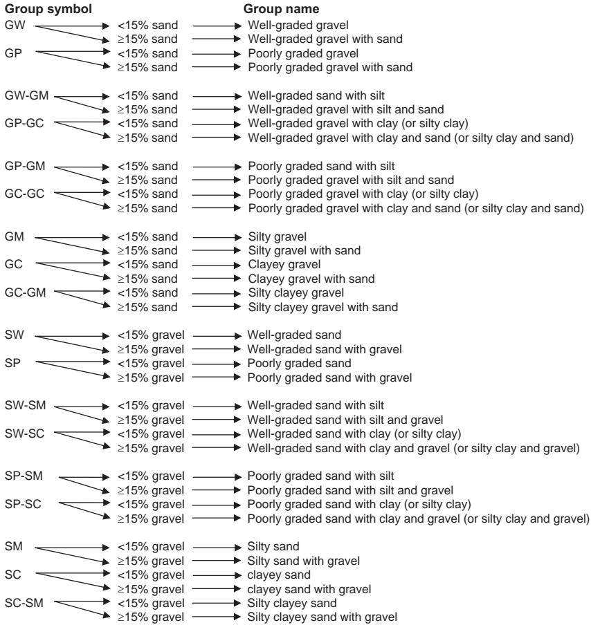
Figure 3.4 Flowchart for USCS classification group names of coarse-grained (gravelly and sandy) soil. After ASTM D2487.
