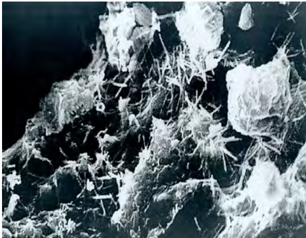
Figure 11.6 Micrograph of a reacted soil-lime mixture. Courtesy of Carmeuse Natural Chemicals.
