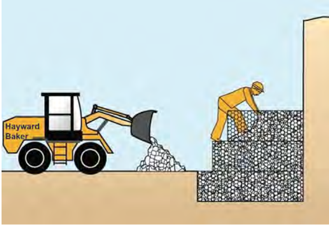
Figure 16.8 Gabion (buttress) retaining wall construction schematic. Courtesy of Hayward Baker.
