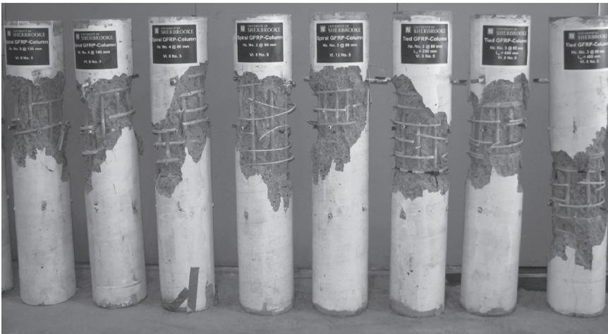
(c) Column specimens after failure
