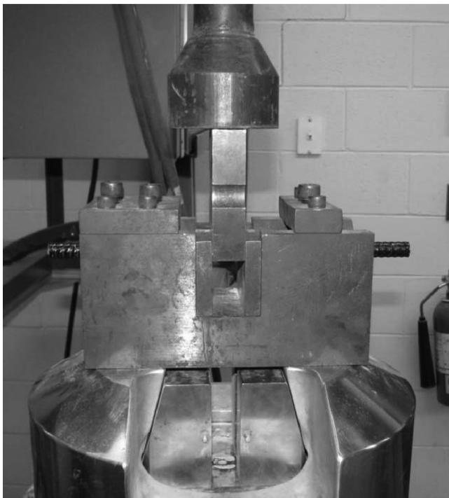
Figure 3.5 Typical transverse shear test setup.
