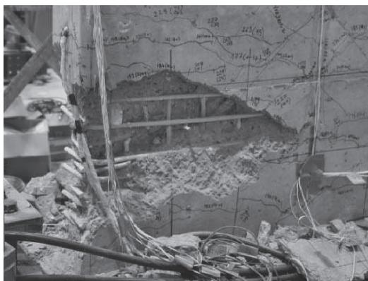
(b) Concrete crushing causing failure
