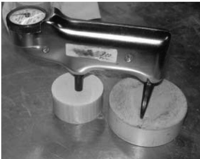
Figure 3.17 Barcol hardness test setup and apparatus.
