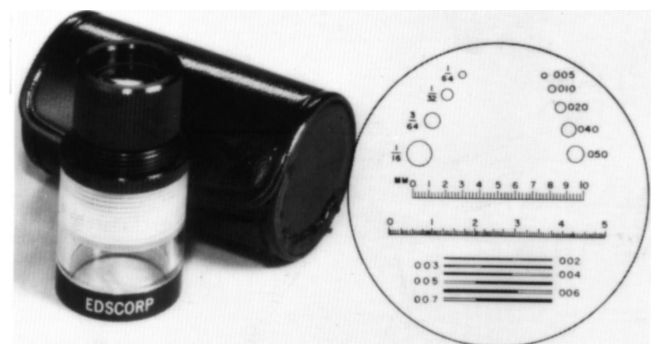
Fig. 2.1-Comparator for measuring crack widths (courtesy of Edmund Scientific Co.)
