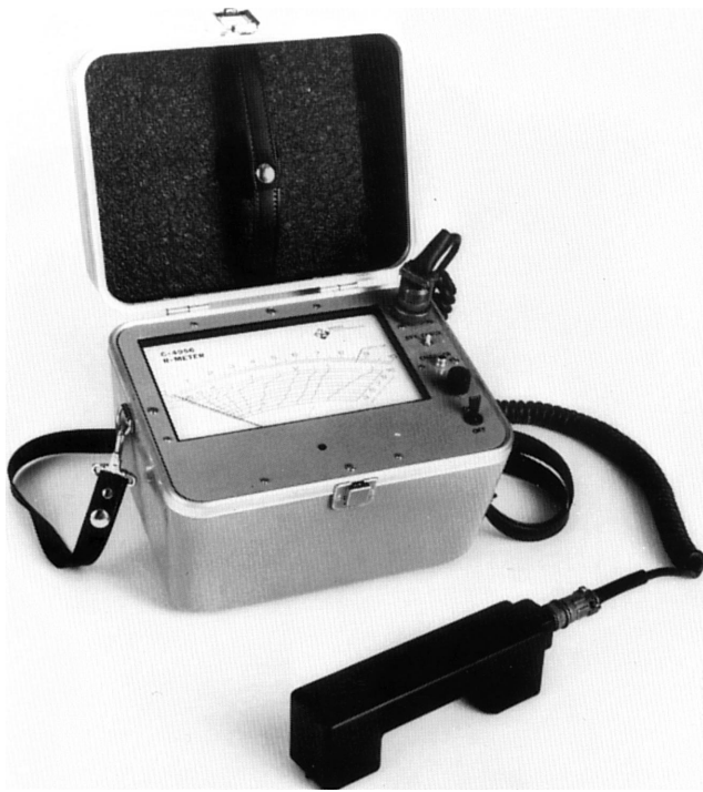
Fig. 2.3-Pachometer (reinforcing bar locator) (courtesy of James Instruments)
