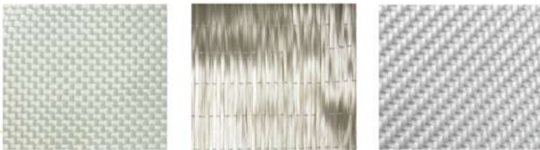
Glass fiber wrap in plain, unidirectional and twill weave
